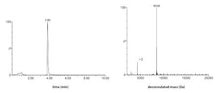
**LC-MS analysis.** Mobile phase A = 1% CH<sub>3</sub>CN, 0.1% formic acid in water (milliQ) and B = 1% water (milliQ) and 0.1% formic acid in CH<sub>3</sub>CN. XBridge BEH300 C18 5µm 4.6x100mm; flow rate = 0.8 mL/min, runtime = 10 min, column T = 40°C. Gradient: 30%  $\Rightarrow$  60% B over 6.5 min.
