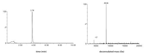
LC-MS analysis. Mobile phase A = 1% CH₃CN, 0.1% formic acid in water (milliQ) and B = 1% water (milliQ) and 0.1% formic acid in CH₃CN. XBridge BEH300 C18 5µm 4.6x100mm; flow rate = 0.8 mL/min, runtime = 10 min, column T = 40°C. Gradient: 30% ⇒ 60% B over 6.5 min.
